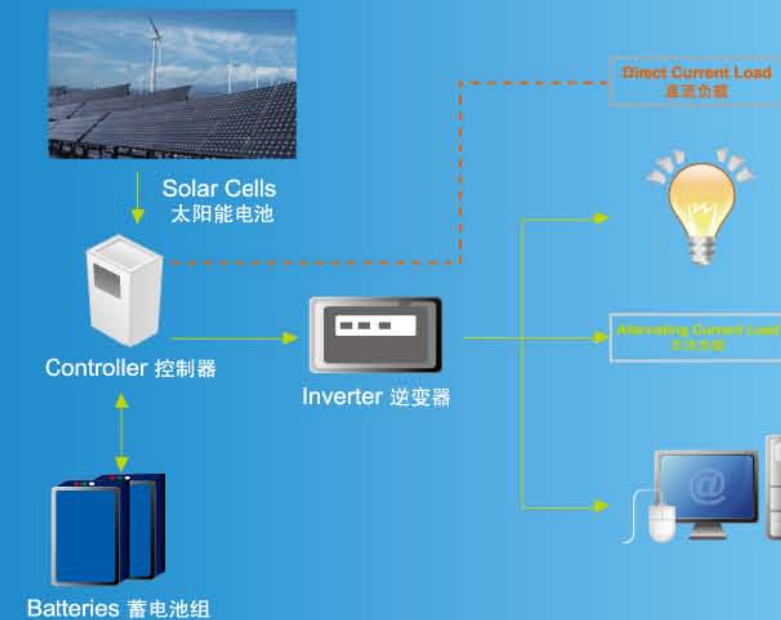
Schematic Diagram of Photovoltaic Power Generation System 光伏发电系统示意图
